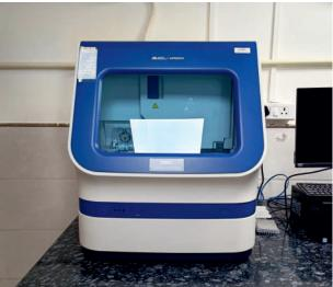
The Sanger Sequencer, developed by Frederick Sanger in the late 1970s, is a crucial tool in molecular biology and genetics. It operates by DNA synthesis using chain-terminating dideoxynucleotides (ddNTPs), enabling precise DNA sequence determination.
